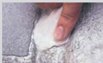
Floor pan holes were repaired with POR-15® Rust Preventive Coating, then pits were filled with Epoxy Putty.
