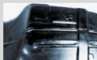
The floor pan was topcoated with Top Coat Chassis Black.
