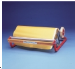
Apron Taper 06865 Dispenses single aprons up to 18 in. wide or any combination of two paper or film widths up to 18 in. wide with Conversion Kit, Part No. 6782.* Film Cutter Blade, Part No. 6785
