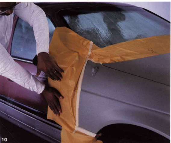
10 Fold 3M™ ScotchBlok™ Masking Paper back onto the 3M Overspray Masking Liquid. Make sure the smooth treated side contacts the masking liquid. Tape tabbing is not necessary.
