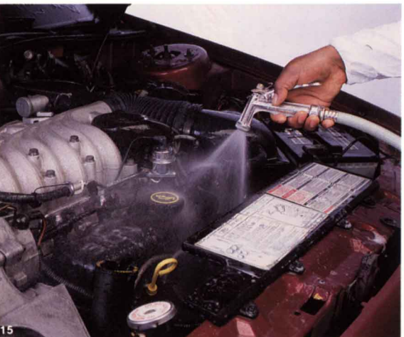
15 Remove the 3M™ Overspray Masking Liquid by rinsing with water from a garden hose or pressure washer.
