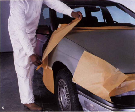
5 Fold the 3M™ ScotchBlok™ Masking Paper back onto the area to be painted and tab with masking tape if necessary.
