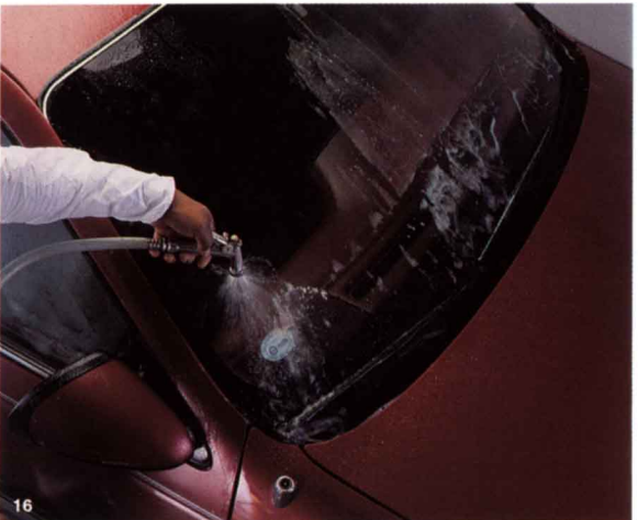
10 Remove any 3M™ Overspray Masking Liquid from the area to be painted by wiping with a damp sponge followed by a dry cloth. Note: Use 3M™ ScotchBlok™ Masking Paper, 36 in. soaked in water to cover tires that are next to the area to be painted.
