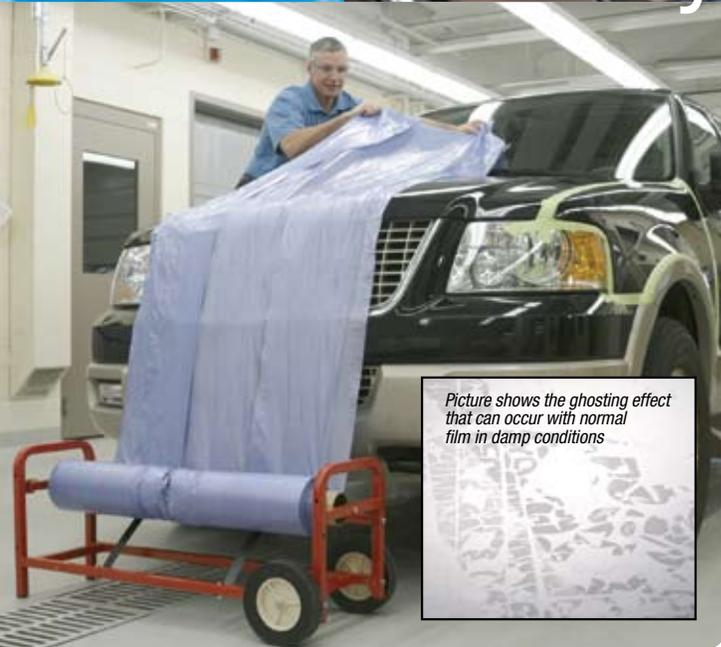
*Picture shows the ghosting effect that can occur with normal film in damp conditions*
