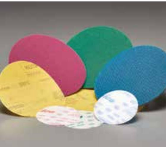
For use on random orbital and rotary sanders. The industry's highest performing film and foam finishing discs are engineered for composite, automotive, and other fine finishing applications. Norton microfinishing film discs produce superior finishes dry without sacrificing cut rate while Norton foam finishing discs are used moist to produce a semi-polished surface to reduce buffing time.
