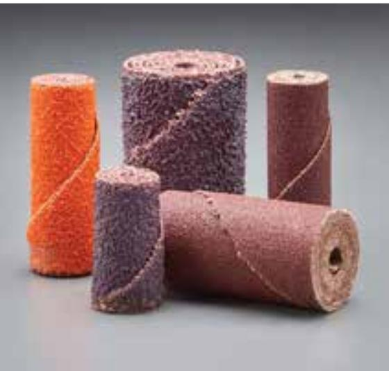
Cartridge rolls are strips of abrasive cloth rolled and glued to form a solid shape that is designed to break down during use and reveal the next layer of abrasive. Valuable abrasive tool for reaching into corners, where larger diameter tools cannot work
