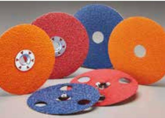
The strongest of coated abrasive discs with resin over resin construction on heavy-duty fiber backing. Designed for applications ranging from heavy stock removal to surface blending. Used with back-up pads on portable angle grinders.
