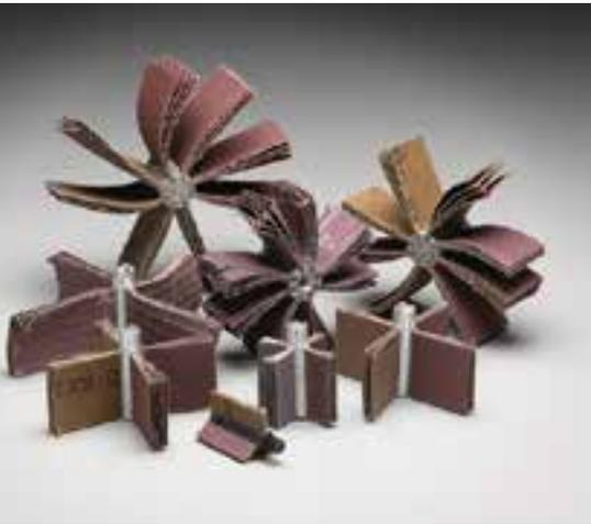
Flaps of abrasive cloth are stacked, inserted into a holder, and then attached to a mandrel. The flaps are designed to break down during use and reveal the next layer of abrasive.
