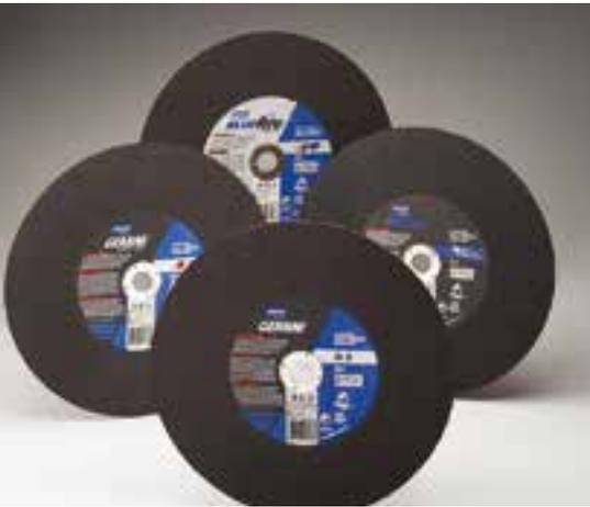
A chop saw is a light, low-horsepower portable machine. Although very similar to a compound miter saw, it is designed for cutting denser materials, like metal bar, tubing or pipe. Chop saw cut-off wheels are designed specifically for this machine with finer grit, softer grades, and reinforcement layers that match the application.
