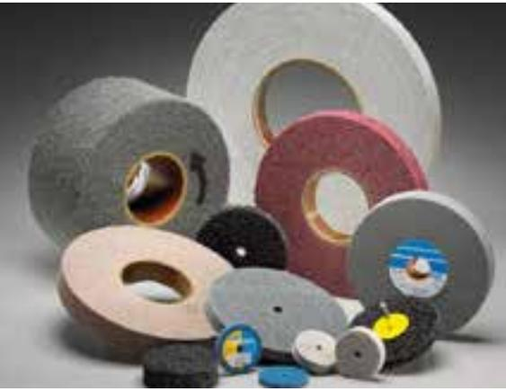
Made from non-woven synthetic fiber mesh, which is impregnated with abrasives and bound with resins, non-woven wheels are designed to create desired surface finish where little or no stock removal is required. The industry's broadest offering is available for light stock removal, deburring, blending, finishing and polishing. Non-woven wheels have an open mesh construction that is waterproof, washable, conformable and non-loading.
