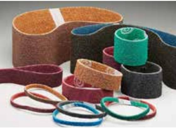
Norton non-woven belts are a combination of strong synthetic mesh and quality abrasive, bonded together by a smear-resistant adhesive. The open construction of non-woven material enables aggressive cutting action and improved surface finish while maintaining its non-loading feature.
