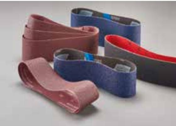
Portable belts are ideal for all your metal and woodworking applications. Choose 36 – 50 grits for rough/heavy-duty applications, 60 – 100 for intermediate, and 100 – 220 for finishing/polishing applications.
