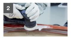
Prepare area with a 3M<sup>™</sup> Roloc<sup>™</sup> Disc P80 reducing the thickness of the plastic.
