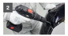
Drill a hole of 4–6mm in diameter at the base of the tear in order to release stress and prevent extension of damage.
