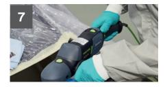
Remove holograms and swirl marks by using 3M™ Perfect-it™ III Ultrafina SE Polish on a Blue High Gloss Pad. Wipe off excess compound using a blue ultra soft cloth.
