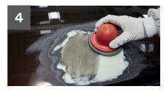
Apply 3M<sup>™</sup> Dry Guide Coat and hand or machine sand the filler to the desired shape.
