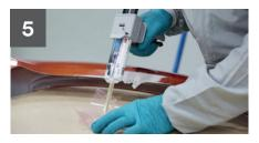
Cut the 3M™ Contour Sheet to about 3 times the size of the tab to be repaired. Equalise and extrude the 3M™ Superfast Plastic Adhesive onto the 3M™ Contour Sheet.
