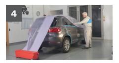
Use 3M™ Masking Film to protect those large areas of the car not to be sprayed during the repair.
