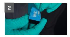
Alternatively, to remove paint imperfections, use 3M™ Paint Defect Removal Hand System, selecting appropriate block size and grade.
