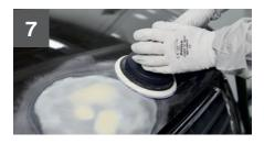
Feather around the repair area ensuring that any deep scratches are removed using a finer grade abrasive.
