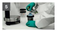
Attach 3M™ PPS™ to gun by aligning the 3M™ PPS™ Lid Legs with the PPS™ adapter and then twist to lock.
