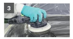
Refine the scratches caused by removing paint imperfections using 3M™ Trizact 3000 Disc wet.
