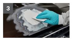
Mix and apply body filler to damaged area, avoiding surrounding paintwork. Reshape panel as required.
