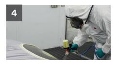
Apply etch primer on any bare metal areas using 3M Accuspray™ Gun and 1.4mm nozzle.
