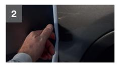
For shallower apertures, use 3M<sup>™</sup> Soft Edge Masking Foam Tape PLUS.
