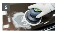
Remove paint from the damaged area using a dual action sander combined with the relevant 3M abrasive, ranging from P80 to P120 grade.
