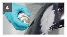
Wipe away dust and debris and apply 3M<sup>™</sup> Polyolefin Adhesion Promoter to both sides of the repair area. Allow 10 minutes to dry.
