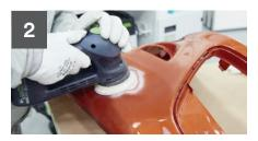
Prepare the area around the damage using a 3M™ Hookit™ Abrasive Disc P180. Avoid overheating and melting the plastic.
