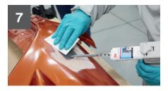
Using 3M Applicator, apply 3M<sup>™</sup> Flexible Plastic Repair Materials to the damaged area. Spread and smooth and allow to dry for 20 minutes.
