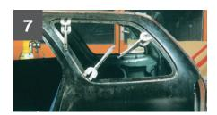
Spray 3M™ Weld Thru II Coating (50410) to all areas to be welded. Clamp the panel in its proper position.
