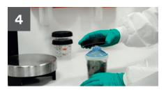
Snap a  $3M^{\infty}$  PPS $^{\infty}$  Lid (with built-in filter) onto the  $3M^{\infty}$  PPS $^{\infty}$  Cup/Liner. Secure the Lid with the locking  $3M^{\infty}$  PPS $^{\infty}$  collar.
