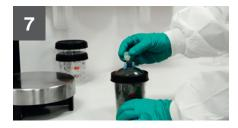
To store colours for future use, insert a sealing cap in the top of the  $3M^{T}$  PPS<sup>TL</sup> Lid.
