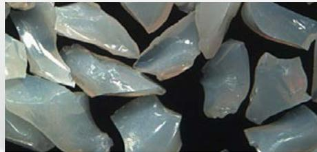
New Norton BLAZE ceramic grain shape is sharper with keener cutting edges that generate a more aggressive yet cool cut.
