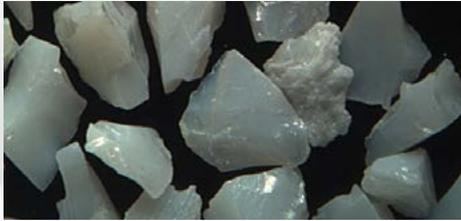
Current generation of ceramic grain shape is blocky with more rounded edges and cuts less aggressively with greater friction.
