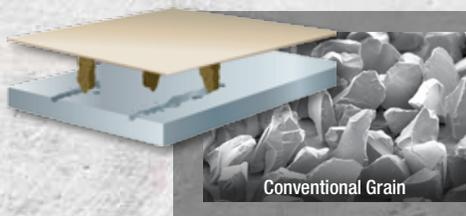
Conventional ceramic abrasive grain is irregular in shape. Instead of a clean, machining action, the grain “plows” through the metal, causing heat build up, slower cutting and shorter life.
