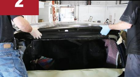
Dry fit all panels to ensure proper alignment. Drill holes or mark locations for:
