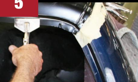
Clamp panel in place. Do not over clamp. Wipe away excess material.
