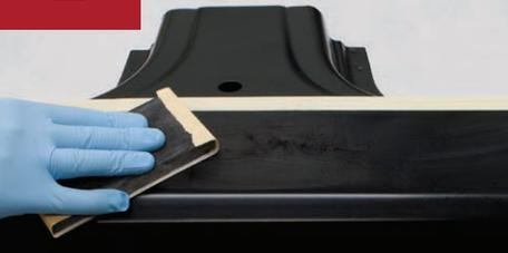
Sand primer with P180 grit. Sand bare metal with P80 grit. Blow off and tack clean. Re-clean with **SEM Solve** or **XXX Universal Surface Cleaner**. Wipe clean in one direction with clean, lint-free cloth.
