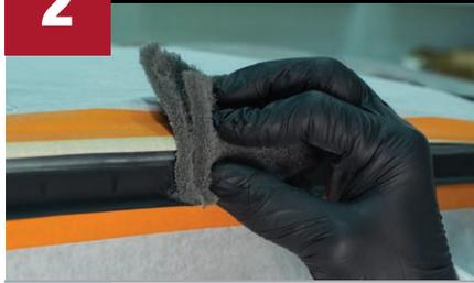
**Bare Metal Surfaces:** Sand with P80 grit. Blow off and tack clean to remove lint and dust. Re-clean with **SEM Solve** or **XXX Universal Surface Cleaner**.
