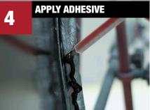
Apply 3/8" - 1/2" bead of **Dual-Mix**<sup>TM</sup> Multi-Purpose Panel Adhesive or **Dual-Mix Weld-Bond Adhesive** to both surfaces. Use enough material to completely fill the joint when parts are clamped. Tool with a spreader or acid brush. Cover all exposed bare metal. (i) For smaller parts use **Dual-Mix**™
