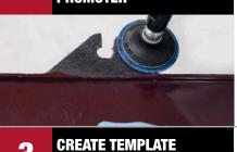
Grind repair on both sides at low RPM or by hand with P36 grit disc. Drill 1/8" holes in repair area to help "lock in" the repair material. Blow off surface.
