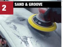
On front side, sand repair area with P80 grit. Dish out damage with P36 grit disc at a low RPM. On back side, grind repair area with P36 grit disc at a low RPM. Blow off surfaces. Re-clean if necessary.
