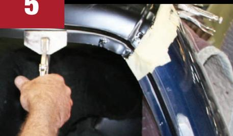
Clamp panel into place. Do not over clamp. Wipe away excess material.
