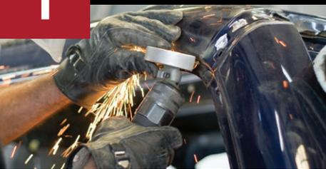
Remove spot welds with spot weld cutter. Remove rivets by drilling or grinding. Remove damaged panel and straighten bent flanges with a hammer and dolly.
