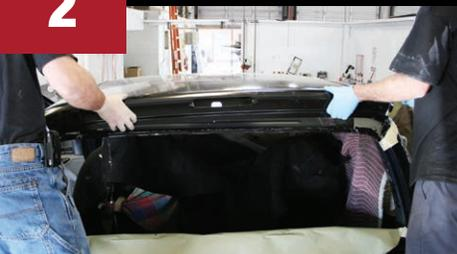
Dry fit all panels to ensure proper alignment. Drill holes for replacement rivets or mark locations of self-piercing rivets.
