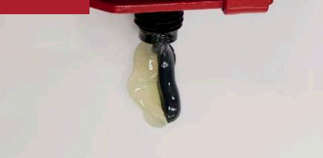
Place **Dual-Mix™ Sound & Seal Sprayable Coating** into **Universal Pneumatic Applicator**. Equalize cartridge until sides dispense equally. Attach **Quick Spray System** to cartridge.
