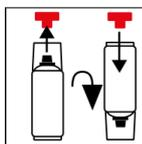
Remove the red button from the cap. Turn the can by 180° and fit the button onto the pin.
