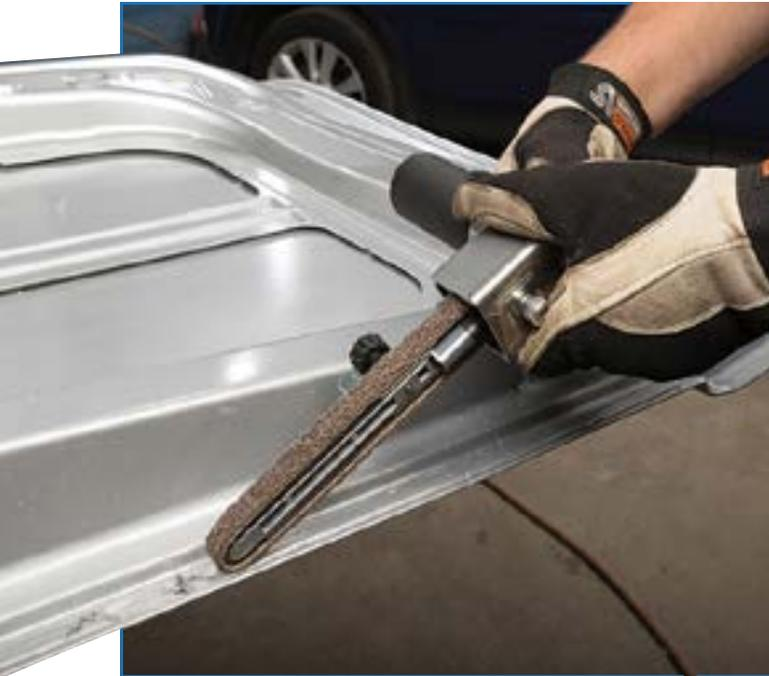
Remove spot welds faster than bits
